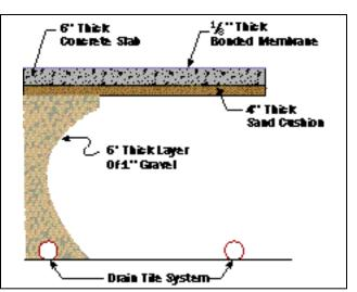
the water table was Figure 4. Swimming pool floor construction details.
