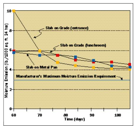
Figure 1. Variations in moisture emission over time for concrete slabs of differing thickness and cast on differing surfaces.
