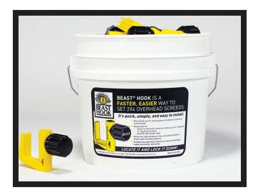
Winner of a 2017 World of Concrete "Most Innovative Product" award, Beast Hook is engineered to hold a 2x4 overhead screed rail in place during concrete placement, replacing outdated cast steel screed hooks concrete placement crews have used for decades. These antiquated metal hooks required additional tools to install and were prone to rusting and stripping of their threads.
