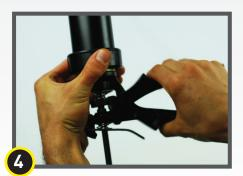
Press the trigger as needed to bring the top of Stego Mastic Sausage Tube to the edge of the gun chamber
