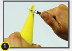
Cut nozzle to the desired width
