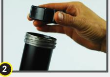
Unscrew the top lid of the mastic gun, push the release mechanism and pull out the metal plunger arm
