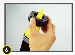
Place the nozzle over the top of the chamber/mastic tube and screw the lid back over and onto the mastic gun
