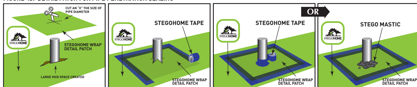
FIGURE 5: MULTIPLE PIPE PENETRATION SEALING
