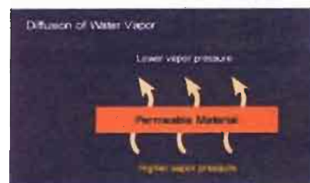
Diffusion of water vapor leads to moisture reaching the slab from below.
